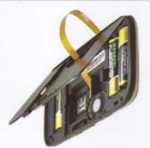
Clip the battery cover back on, the ribbon cable will fit in a small opening allowing it to come through the cover.
