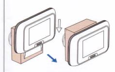
Taking extra care with the ribbon cable gently push the indoor monitor (A) back onto the steel bracket (D) and slide down to lock into position
