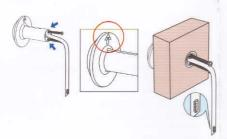
Insert your selected screws (B) according to your door thickness into the Outdoor camera (C) but do not fully tighten
