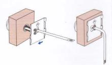
Using the steel bracket (D), make sure the up arrow is facing up and push the ribbon Cable through the slot. Then allow the screws to push through the holes so the steel bracket become flush with the door
