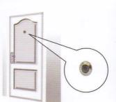
Either remove your current door viewer or drill a new hole at least 13mm diameter up to 20mm diameter Into your door in a suitable
